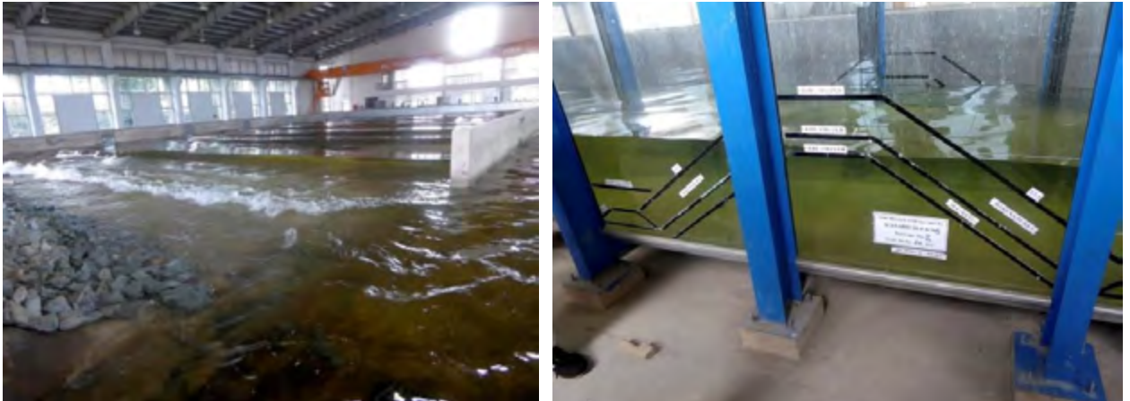
Fig. 36. Left: Wave basin in the experimental hall with wave generator and riprap absorber. Right: Wave flume tank at the Southern Institute for Water Resource and Research SWIRR. These facilities are very suitable for physical testing of scale models of different waterworks. Source: Holger Schuettrumpf & Peter Froehle
