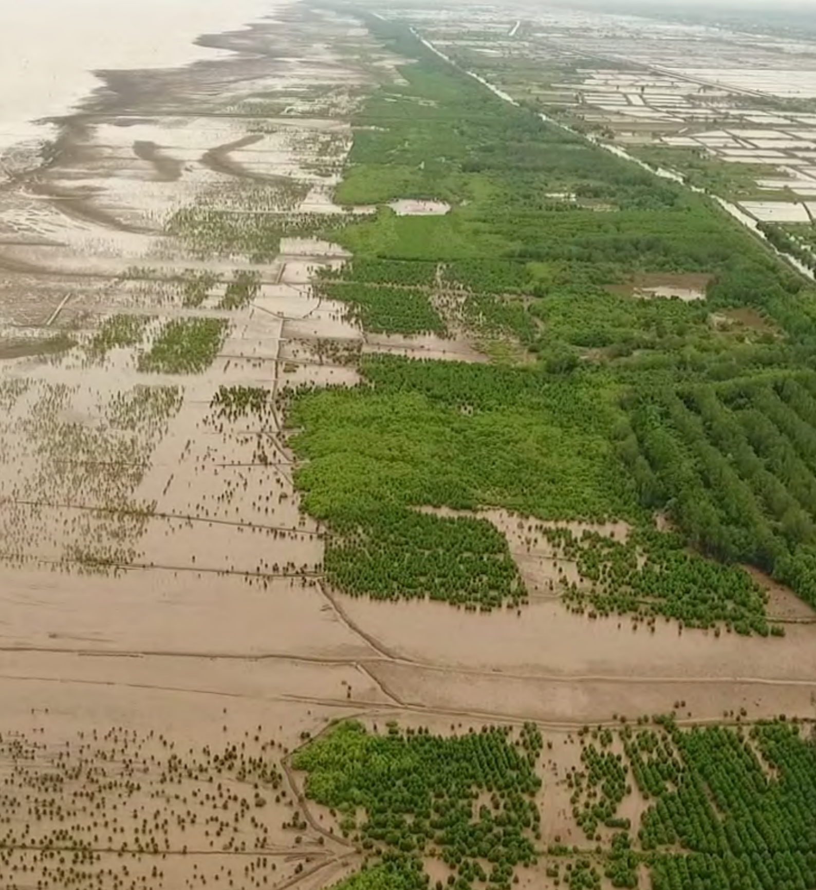
Fig. 2. Still picture by a drone (UAV) from the coast of Soc Trang at low tide. On the right side, aquaculture ponds are encroaching close to the sea-dyke. There is a channel in front of the dyke which was ditched during the construction of the dyke. Reforested mangrove plantations of different ages are covering the upper intertidal area, which falls dry at low tide. On the seafront, one can recognize undulating sediment accumulations and some probably wild recruitment of mangroves. One can also see marks of fishing gear on the lower tidal mudflats. Source: Soc Trang Department of Agriculture and Rural Development
