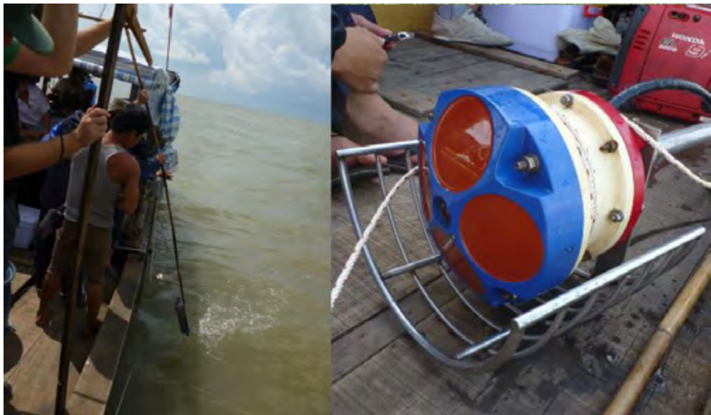
Fig. 6. Sediment sampling (left photo) and measurements on currents and wave regime with an ADCP (Acoustic Doppler Current Profiler, right photo) in West and East Sea around Ca Mau Province. Source: Stefan Groenewold
