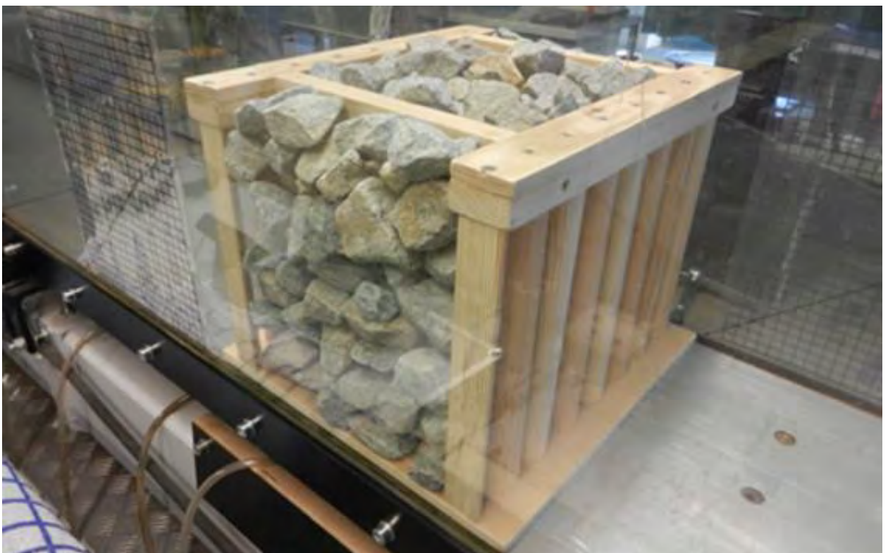
Fig. 37. Physical model of riprap pillar construction (as used in Ca Mau, West sea) in the flume tank of the Technical University of Hamburg-Harburg, Germany (TUHH). The system of Ca Mau's breakwater was reproduced at a reduced scale of 1:10 in the laboratory and the hydrodynamic forces were represented in correct proportions to the actual system. The transmission coefficient and other parameters could be determined and combined with field studies on sediment accretion and resulted in the recommendation to develop some modifications. Source: Philipp Jordan
